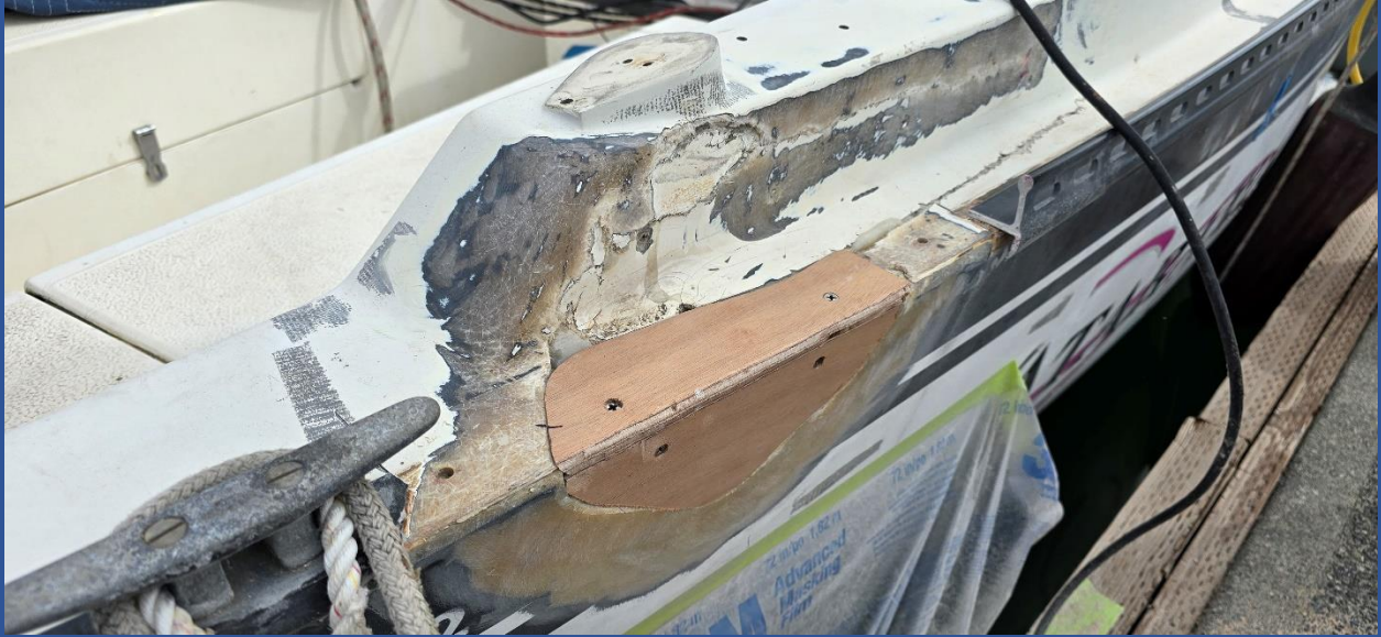
Coaming damage pulled out and glassed from inside; wood pieces fitted
