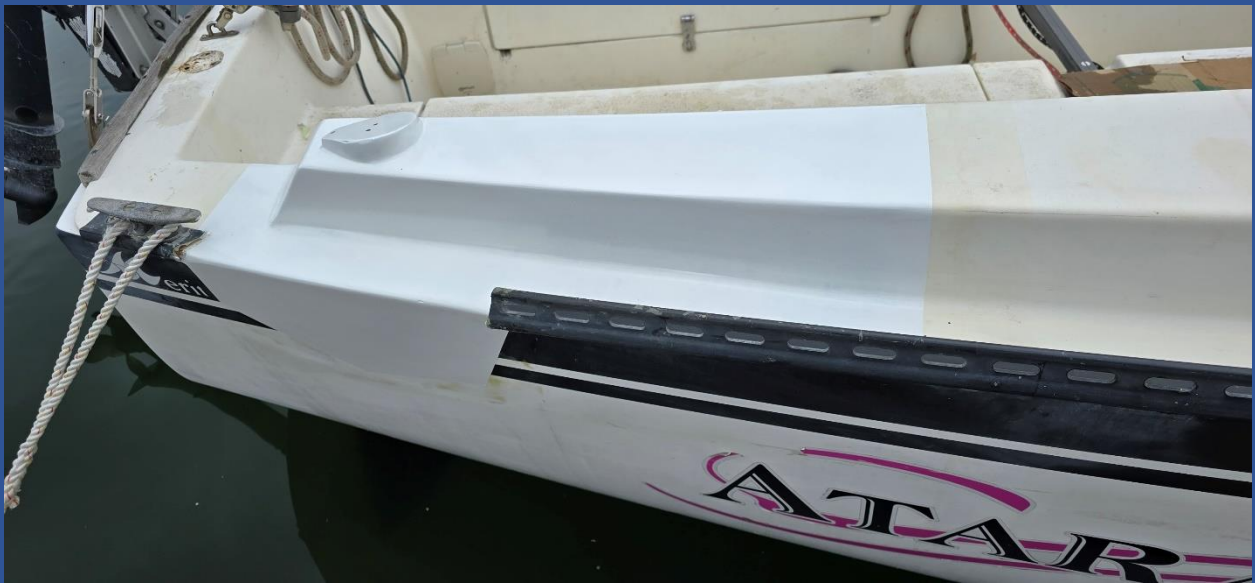
Several layers of fiberglass inside and out; faired; and painted.
